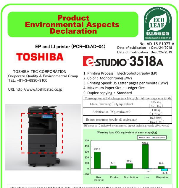
The above environmental load is calculated assuming that the usage period is 5 years and the total number of printed sheets is 735,000 pages. Also, the printing paper is not included in the calculation range. Outside the red frame of the photo is not included in the LCA calculation because it is the accessories (document feeder and paper feed unit).
