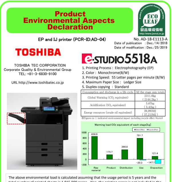
The above environmental load is calculated assuming that the usage period is 5 years and the total number of printed sheets is 1,815,000 pages. Also, the printing paper is not included in the calculation range. Inside the red frame of the photo is not included in the LCA calculation because it is an accessory (paper tray).
