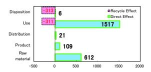
Use stage: Printing 1,215,000 A4 sheets in 5 years. The environmental load of sheet in "Use" stage is not included in above data.
